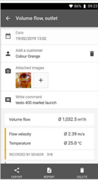
The screenshot shows a mobile application interface for a measurement. At the top, it displays the date and time: 19/02/2019 13:02. Below this, there are sections for adding a customer (Colour Orange) and attaching images. A comment section notes the 'testo 400 market launch'. The main data area shows measurement values: Volume flow (Ø 1,032.5 m³/h), Flow velocity (Ø 2.39 m/s), and Temperature (Ø 25.0 °C). At the bottom, there are buttons for EXPORT, REPORT, and DELETE.
